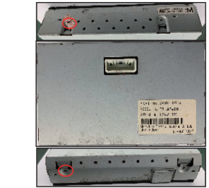
1, Unscrew 4pcs screws to open the back cover
